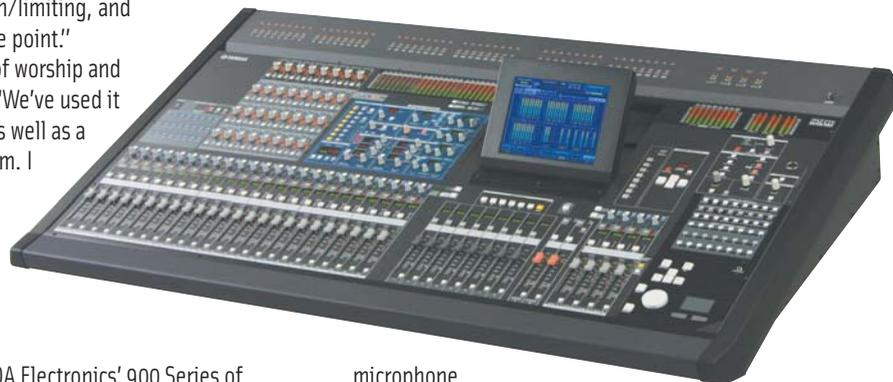
microphone preamps, plus an additional four stereo line level inputs. The PM5D-RH includes 48 XLR analog mono inputs with recallable microphone preamps, with four stereo inputs that accept mic level signals. The console offers 130 input connections and can simultaneously mix up to 64 inputs to stereo or LCR stereo. The PM5D provides 24 mix buses, onboard DSP, and 500-scene total recall capability.
