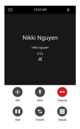
You can also view active and held calls in progress on the system, as shown next. Swipe the screen from the bottom to the top to view all the calls on the system. If the system has multiple lines, active and held calls display under the associated line.
