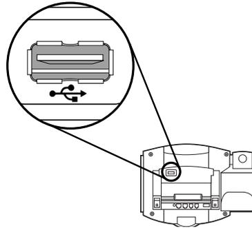
When you plug in the USB device, the USB device is supported and the message “USB device attached.” appears or the USB device is tested to determine if it is acceptable. If it is accepted, the message “USB device attached.” appears. If it is not accepted, the message “Unsupported USB device attached: Go to [www.polycom.com/usb\\_support](http://www.polycom.com/usb_support).” appears. Contact your system administrator about receiving another USB device.
