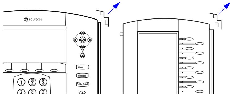
2. Align the SoundPoint IP Backlit Expansion Module at the top of the groove lines on the SoundPoint IP 650 phone and slide it downwards until it clicks into position.
