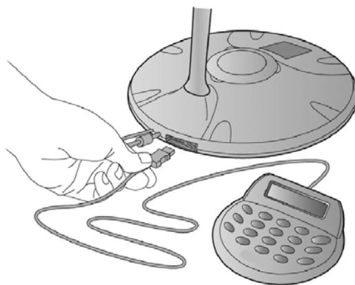
**Figure 13. Connecting external dial pad**
