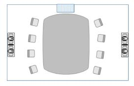
**Scenario 3**: One camera is positioned on the left front of the room and the other is positioned on the right front of the room. This configuration works well in classrooms or large seminars.
