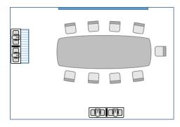
**Scenario 2**: The cameras are positioned at either side of the room with the system at the front. This configuration works well in classrooms or large seminars.
