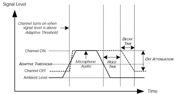
Figure 22. Automixer parameters.
