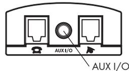
The setting for auxiliary audio needs to match the kind of device that is being connected to the phone.
