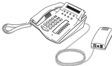
Any digital phone supported by your telephone network can be connected to the phone jack on the Interface Module.
