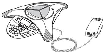
3. Plug the other end into the slot under the SoundStation2 Console as illustrated. Then thread the cable through the channels on the underside of the console as shown at right.
