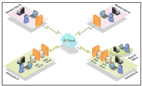
Users in enterprise A and B can place calls to remote user A and B. The remote users can call each other as well as users in both enterprises.
