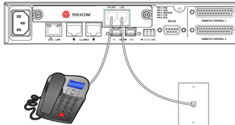
When the SoundStructure TEL1 device takes its *LINE* interface off-hook by using the SoundStructure API (See the SoundStructure Command Reference manual) `phone_connect` command, the audio from the telephone *LINE* interface is routed through the SoundStructure TEL1 and into the
