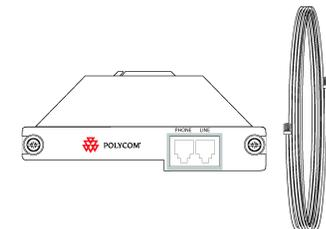
The SoundStructure TEL2 package includes the TEL2 plug-in card and two 15-foot long telephone cables as shown in the following figure.
