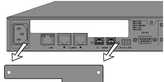
3. Insert the plug-in card into the slotted rails and push until it is tight into the slot.
