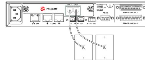
Note that the TEL2 interface does not support an optional handset - both telephone connectors on the rear of the TEL2 are to be connected to analog telephone lines.
