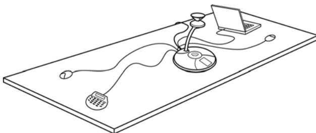
**Figure 12. External dial pad and satellite microphones**
